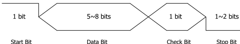
Figure 8.24 Schematic Diagram of RS232 Protocol
