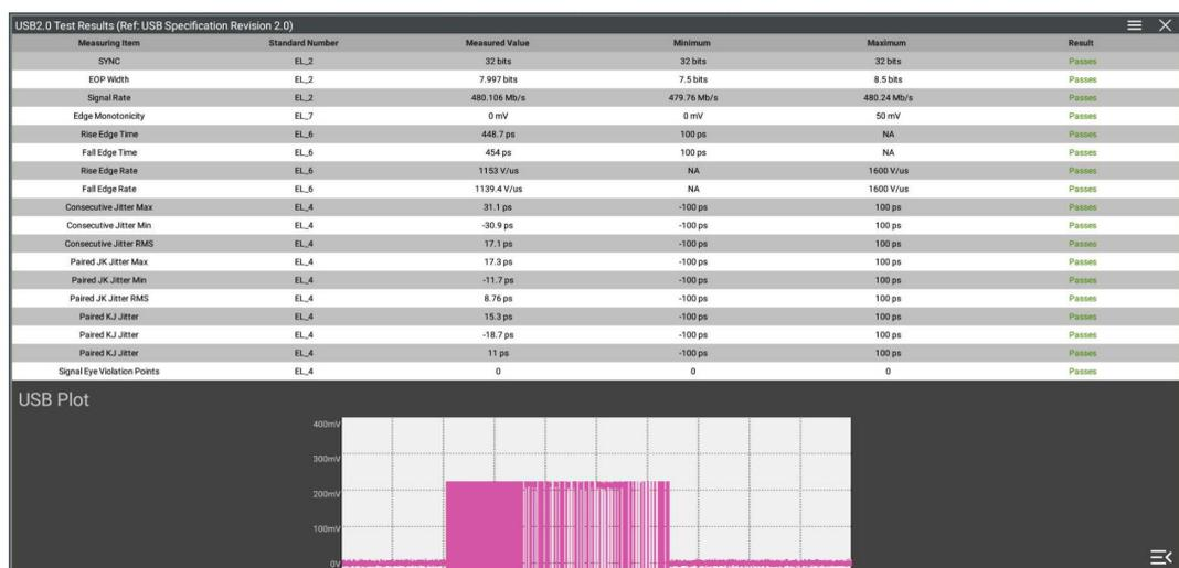
Figure 18.2 USB2.0 Signal Quality Compliance Analysis Test Result
