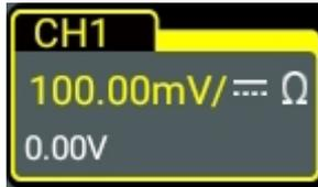
The information displayed in the channel status label is related to the current channel setting (irrelevant with the on/off status of the channel). After the channel is turned on, modify the parameters such as the vertical scale, horizontal time base, trigger mode, and trigger level according to the input signal for easy observation and measurement of the waveform.
