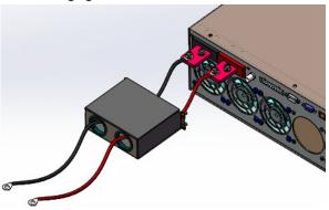
3. Mount the protective covers to the two input terminals.
