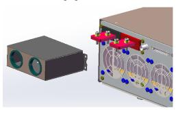
2. Connect the cables to the two input terminals, as shown in the following figure.
