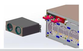
Connect the input cables to the terminals as shown in the following figure.
