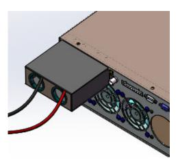
4. Connect the other end of the cables to the DUT. The red cable is connected to the positive electrode and the black cable is connected to the negative electrode.
