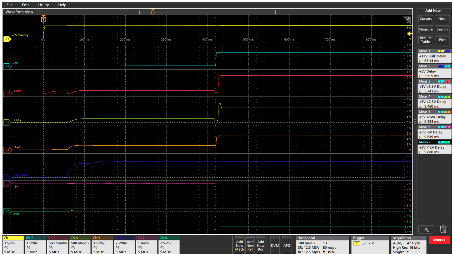
Using automated measurements to characterize power supply bring up.
